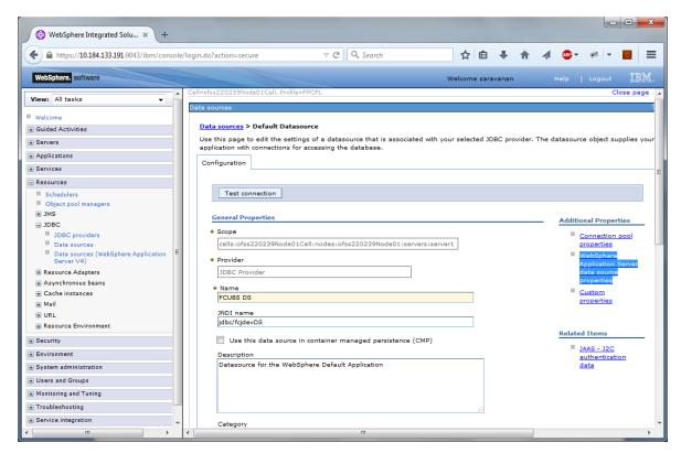
24. Make sure that the checkbox "Use this data source in container managed persistence (CMP)" is unchecked. Then click on the link "Webpshere Application Server data source properties" on the right side.
